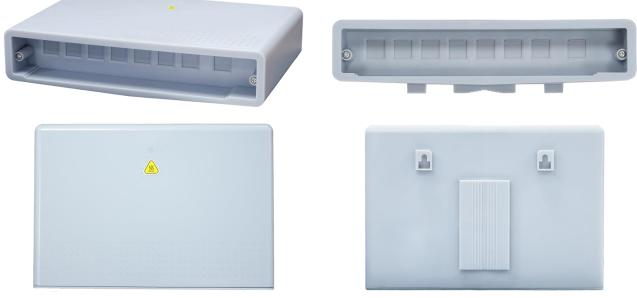
The **ES-7226PoE** is a RMDU (Reverse Multi Dwelling Unit) with eight GE ports. It uses RPU (Reverse Power Unit) powered by 7 PoE (PD) devices from PoE injectors at subscribers' homes. Dynamic load sharing occurs among the PD ports. It also provides one PoE (output PSE) connection to an ODU (5G Outdoor Unit) for Fixed Wireless Access (FWA) or a Fiber ONU, optimizing broadband uplink efficiency.
